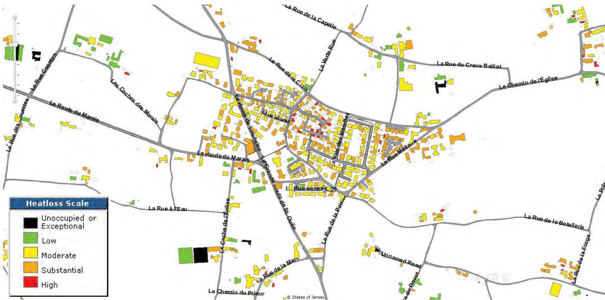
Heat Loss Map - A survey was taken of all Jersey using thermal images taken from aircraft to form a heat map. The information has been distilled into categories of heat emission indicating energy efficiency.
