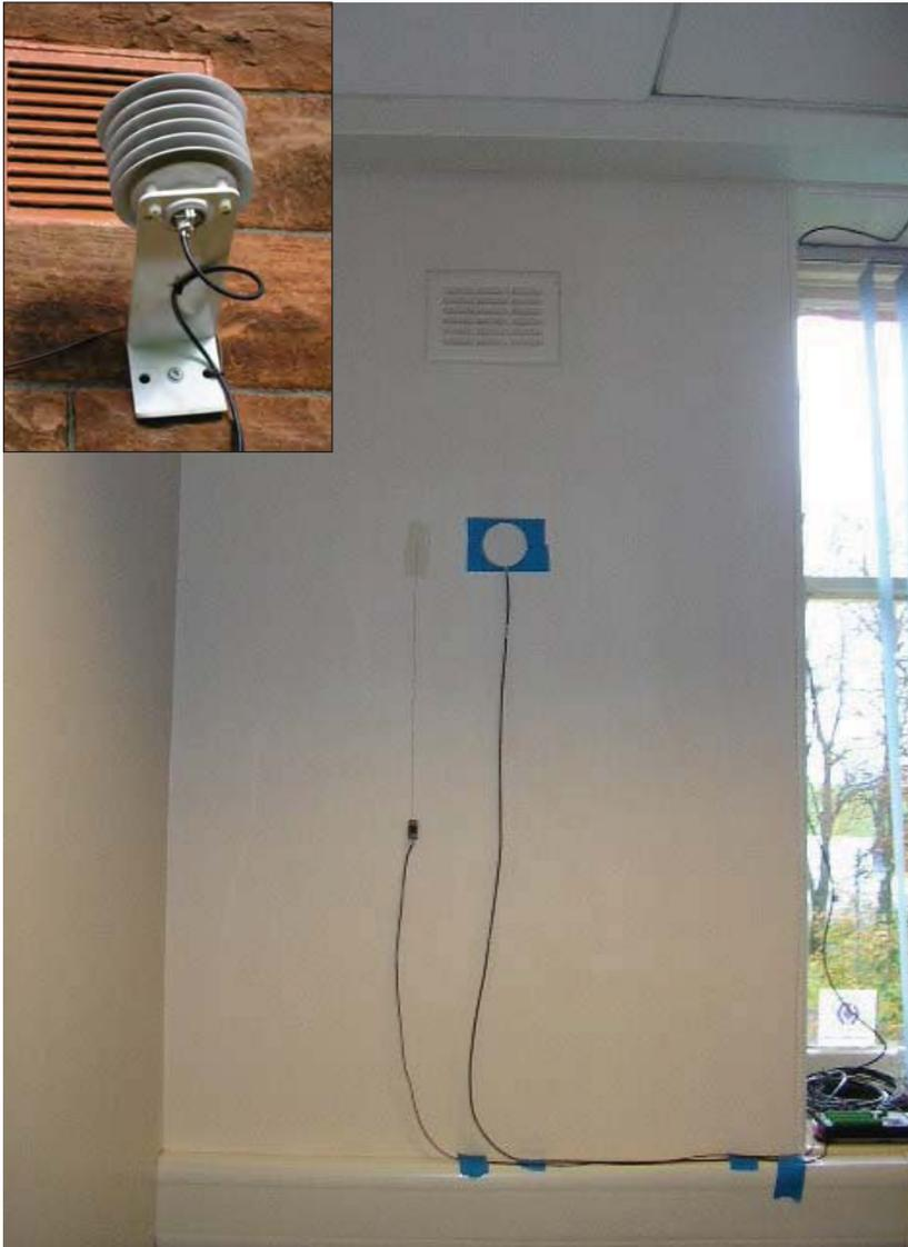
Example Internal Surface Temperature Sensor and External Air Temperature Sensor; reference, Historic Scotland Technical Paper 2 2008
